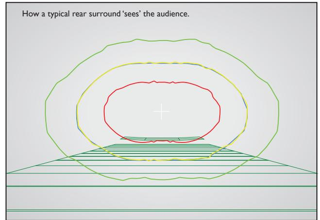
The resulting coverage map of a 7.1 rear surround array is shown bottom left. It has a severe rearward bias and a 7dB differential between front seats and rear seats i.e. the front 1/2 of the theater receives no intelligible rear content. In addition, there is a 4dB differential between the rear row and calibration row. Evaluating the +/-1dB channel balance for all loudspeakers is now restricted to the box shown or 7% of the audience!
