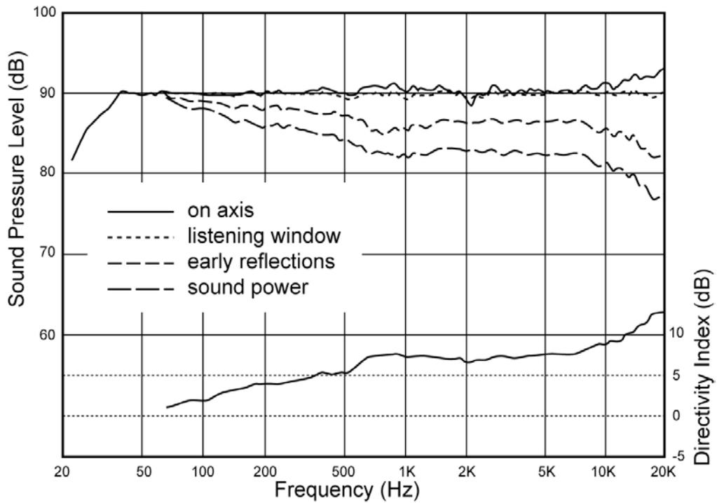
Figure 3 The so-called spinorama of the JBL M2 after it's been measured in the anechoic chamber. The set of frequency response curves represent the quality of direct sound produced by the loudspeaker for
