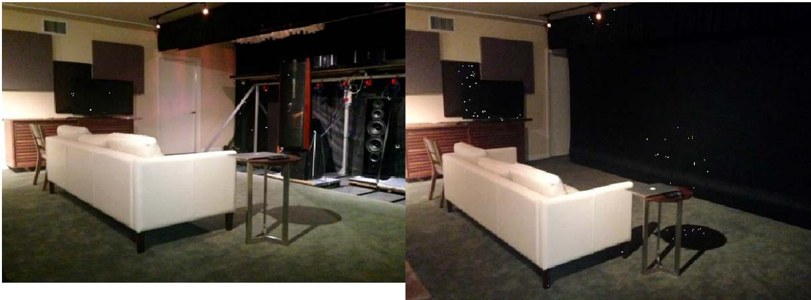
Figure 1 Hundreds of loudspeakers have been subjectively evaluated in Harman's multichannel listening lab (MLL) where listeners make double blind comparisons of different loudspeakers in the same position via an automated speaker shuffler. Important listening test nuisance variables like sighted biases, relative loudness differences, and loudspeaker/listener position are controlled or removed from the test.
