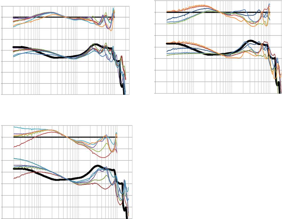
Figure 4 The frequency responses of 15 in-ear headphones plotted in three categories of sound quality (good, mediocre and poor) based on preference ratings of listeners [24]. At the top of each graph is the error response curve: the difference in frequency response between the headphone and the preferred Target curve.
