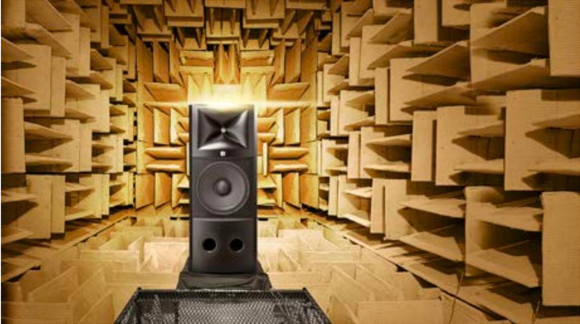
Figure 2 Acoustic measurements of the loudspeakers like the JBL M2 monitor are measured in the large anechoic (reflection-free) chamber at the Harman Acoustic Laboratory in Northridge, California. The acoustic measurements allow accurate predictions of listeners' sound quality preferences in listening rooms.
